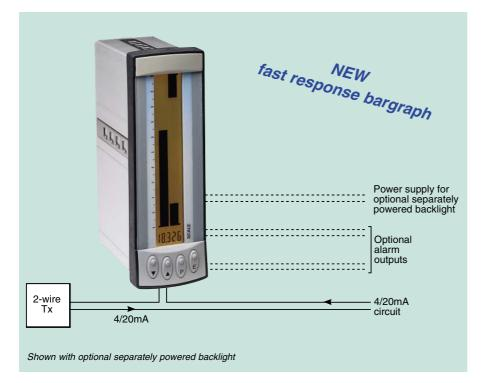
The BA526C is a new combined analogue and digital indicator which replaces the BA526. It offers enhanced features and improved visibility in a shorter enclosure. Like its predecessor, the BA526C displays the current flowing in a 4/20mA loop on a 100 segment bargraph and in accurate engineering units on a digital display. The instrument is loop powered but only introduces a 1V drop allowing it to be installed in series with almost any 4/20mA loop.
